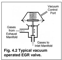
Although EGR is effective, the reduced peak pressure requires that the throttle will have to be opened further to maintain the same level of torque from the engine, an action which will itself tend to increase NOx. Emissions engineers therefore have to carefully juggle conflicting requirements.
