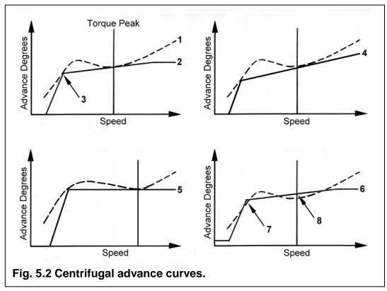
The compromises will be obvious and clearly a centrifugal setup that gives more advance above peak torque speed (better for power) must mean less below. In effect the main advance slope can be considered as able to pivot around the maximum safe advance at the peak torque speed to bias the timing to favour either low speed or high speed operation, but not both.
