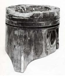
Fig. 5.1 Piston damaged by detonation.
