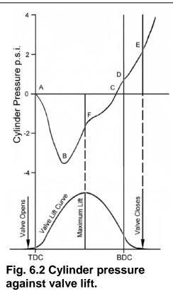
around -8 p.s.i. Another factor is that pulse dynamics (to be discussed shortly) rely on changes of density so can achieve increased mass flow without increasing gas velocity.
