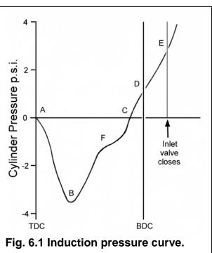
approaching its maximum velocity so the pressure starting to rise again is evidence that the inward flow must be accelerating rapidly as a result of the initial depression.
