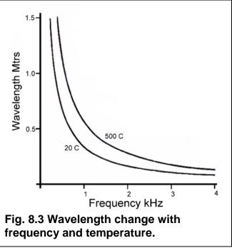
A reflective silencer will therefore be effective over different frequencies when an engine is idling than it will at full throttle. This can explain puzzling anomalies like how an exhaust system can seem to be reasonably quiet whilst being driven under load yet unpleasantly loud when the engine is idling.
